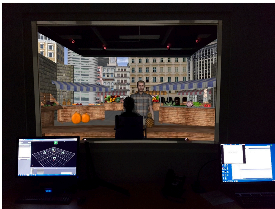
Fig. 4. A virtual reality CAVE setup, as seen from the control room situated behind it. In the CAVE, the participant wears 3-D shutter glasses to become immersed in a virtual environment that is projected around them on large digital screens. In this example, bilingual participants are stand owners at a 3D market place. They communicate with life-size virtual customers in one language or another as a function of the customer's language background (cf. Titus and Peeters, under review).
